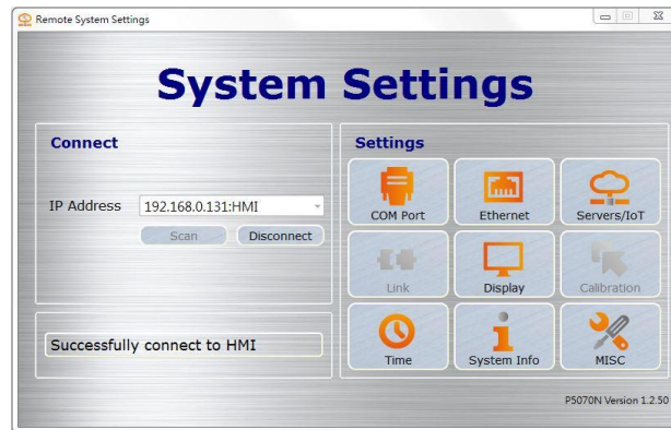
Figure 445 【 Remote System Setting 】 successfully connect to HMI
