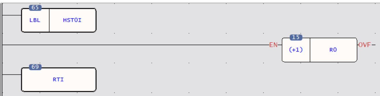
Figure 9 The interrupt sub-program example of cyclic pulse
