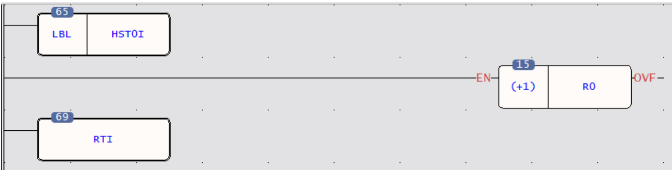
Figure 37 Interrupt subroutine of cyclic pulse
