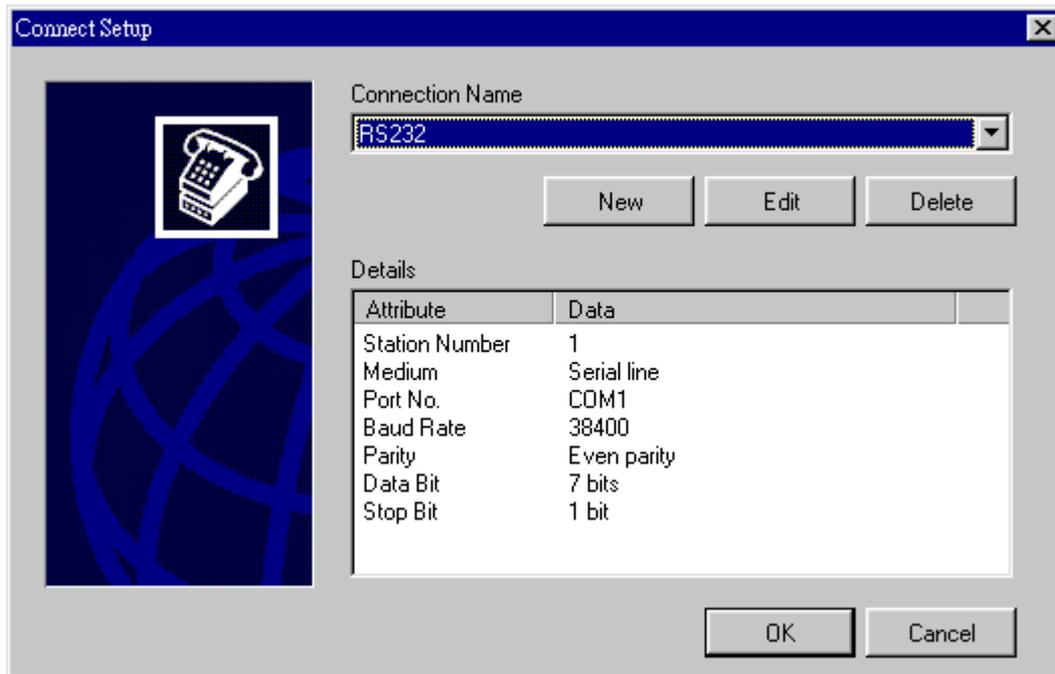
There are three pre-defined connection sessions can be found in the 'Connection Name' combo list which are RS232, UDP, TCP. In this tutorial we assume to connect the PLC with serial line so we can pick RS232 or create a new session with click the [New](#) button which will bring out an wizard to direct you to create a new session. If you don't want to create a new session but the pre-defined session is not exactly what you want then you can click the [Edit](#) button to change it.
