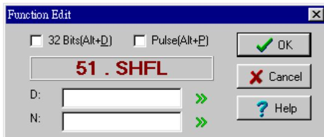
Use mouse to click the check box of Pulse to check it ( to make this function pulse activated) then complete the input of D: and N: field. If you do not know or forgot the meaning of D: or N: filed can move the pointer above the filed name you questioned then there will appear a hint. Also if you forgot the valid input range or data type of specific field you can move the pointer to that input field and there also will appear a hint about the valid data type and range .
