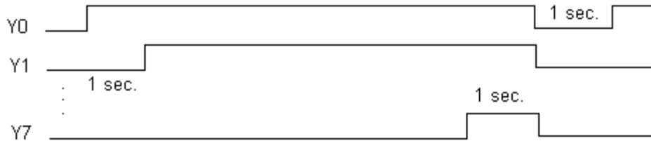
At first Y0 will be 'on' for one second. After that Y1 will also 'on'. This will cycle to Y2 then Y3 ... After Y7 is 'on', the next time all output will all be 'off' for 1 second. This procedure will repeat again as described above.
